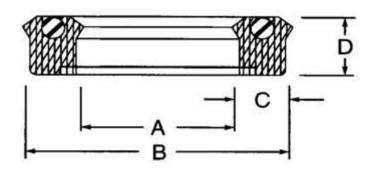
Type "B" loaded lip seals with integral back-up rings can be used when excessive pressures or clearances cause standard rod seals to extrude. Because the back-up ring is "built in" to the seal, these seals will retrofit standard grooves. Also, time and money can be saved by cleaning up scored rod glands and using this seal and a wear band in place of the machined-out metal surface.
