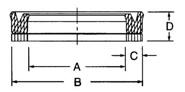
This sealing set is designed to resist extrusion even with an excessive clearance gap. The seal is made from 90+ Shore A hardness urethane and the backup ring is machined from bronze filled TFE or molded from 55 Shore D hardness hytrel.
