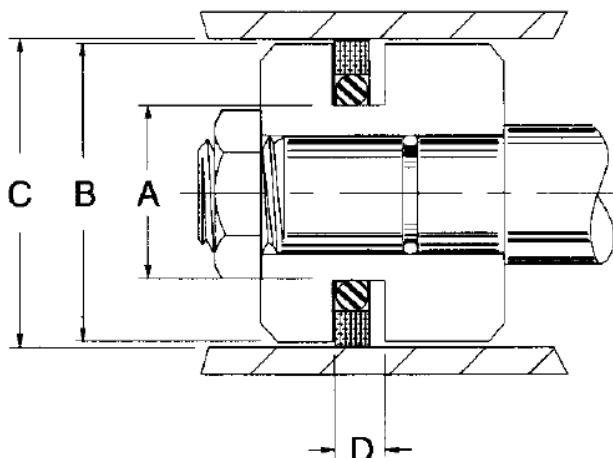
AS800 style square piston seal assemblies are made from glass filled TFE and include an o-ring energizer. This popular medium duty assembly assures dependable service to a wide variety of sealing applications from rotary swivels to reciprocating cylinders.
