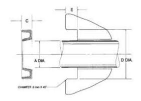
AM45 series wipers are predominately used as grease seals for hinge pin applications in heavy equipment. They are typically lighter duty seals and are not normally used as reciprocating wipers.
